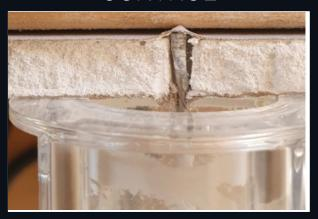
Depth of bit can be set to have bit end penetrate wallboard and not damage framing of items behind wall lining
